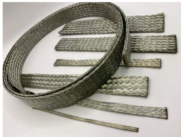
The braids listed are flat tinned copper braids. However Alco manufacture any size and construction of braid. Specialist materials are available including stainless steel, aluminium and nickel plated copper. Alco offer PVC covered flat braids to customers specification. When purchasing PVC covered braid, please allow a reduced current rating of 10%.
